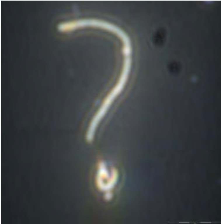
SWNT-H 2 SO 4 Dispersion imaged on Cytoviva Microscope
